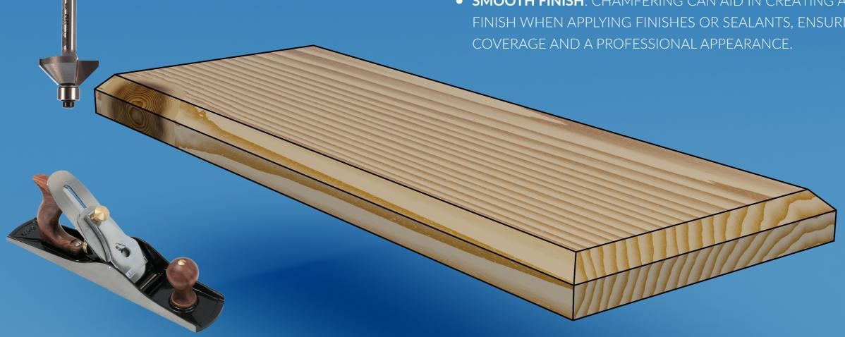
USE A HANDPLANE OR ROUTER TO CUT LARGER CHAMFERS OR SANDPAPER AND A SANDING BLOCK FOR SMALL CHAMFERS.
